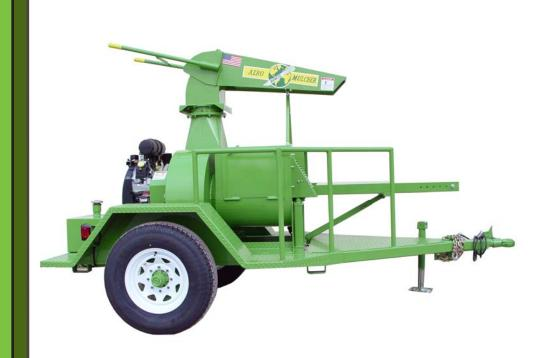
The **Bowie SG-50** is the intermediate workhorse of our manufactured Aero-Mulchers. This unit is powered by a 38 hp Kohler air cooled gas engine to give years of trouble-free service. The discharge gun has a full 360° horizontal rotation and the fan is dynamically balanced. The six (6) blade 23" fan will generate an airflow of 4500 CFM at a velocity in excess of 120 MPH. The feed tray is fully adjustable with a detachable extension. This unit comes as either a skid or trailer mounted.
