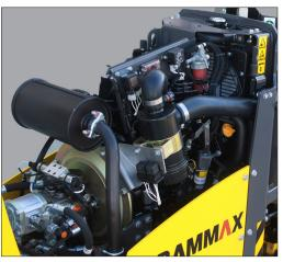
A highly fuel efficient Yanmar engine idles automatically after 15 seconds of no load. Operating run-time can reach up to 11.5 hours with a 7.4 gallons diesel reservoir consuming only 0.74 gal/hr.
