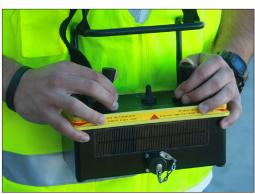
Infrared (IR) control system optimized for both operator safety and functionality. Requires visual contact with the machine for operation. Simplify fleet management by pairing transmitter to roller in seconds via cable connector. Blocks out signals from other machines on the job.
